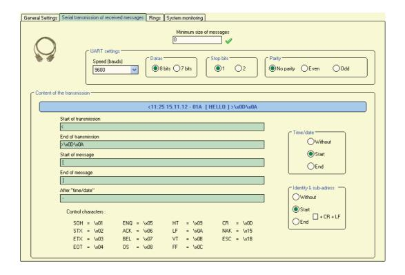
This tab enables to configure the serial output and the text format.
