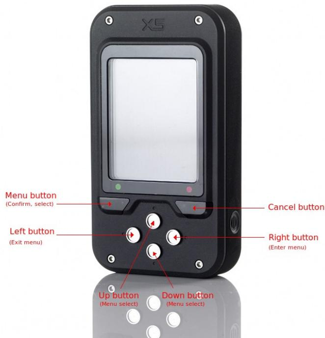
Figure 4: The Buttons on the X5
